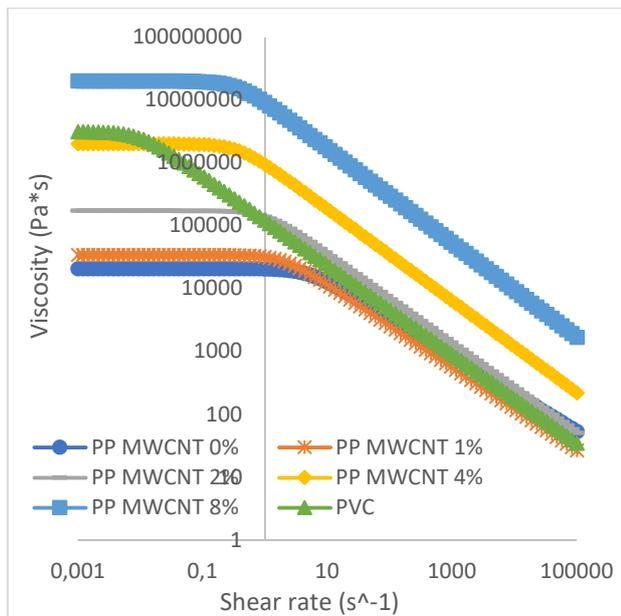
**Figure 3** - Viscosity of PP with varying MWCNT contents and PVC as a function of shear rate.
