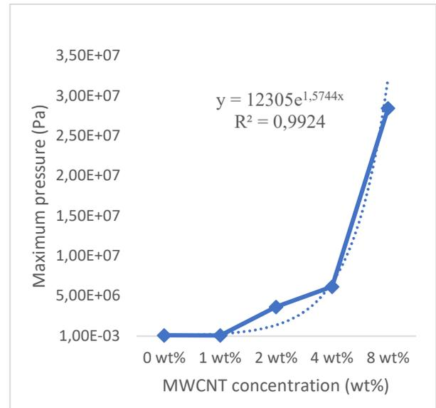
**Figure 8** - Dependence of maximum pressure at the end of the head on MWCNT concentration
