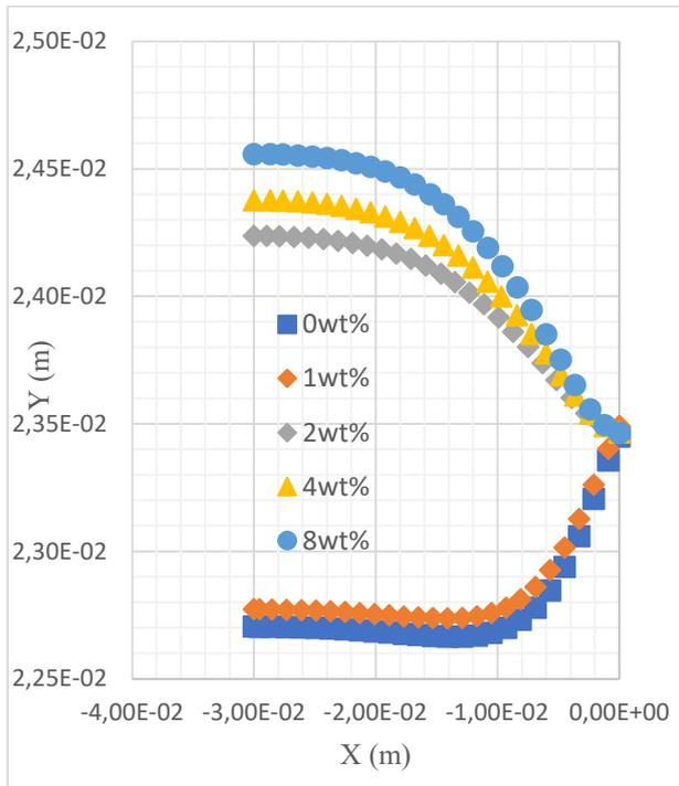
**Figure 12** - Profile of the interface line between PP/MWCNT and PVC layers in the two-layer pipe for different MWCNT concentrations in the local coordinate system
