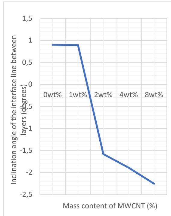
**Figure 13** - Dependence of the inclination angle of the interface line between layers on the MWCNT concentration in the PP/MWCNT composite
