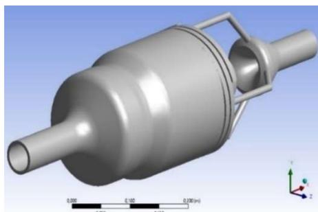
**Figure 1** - Three-dimensional model of the internal cavity of the two-layer extrusion head.
