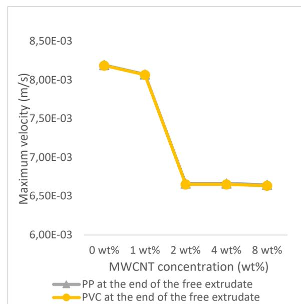
**Figure 10** - Dependence of maximum flow velocity of PP/MWCNT and PVC layers on MWCNT concentration at the end of the extrudate
