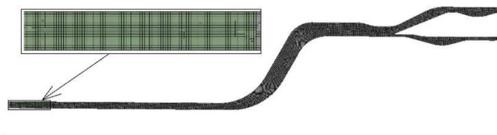
**Figure 2** - Discretization of the cross-section of the studied extrusion head.
