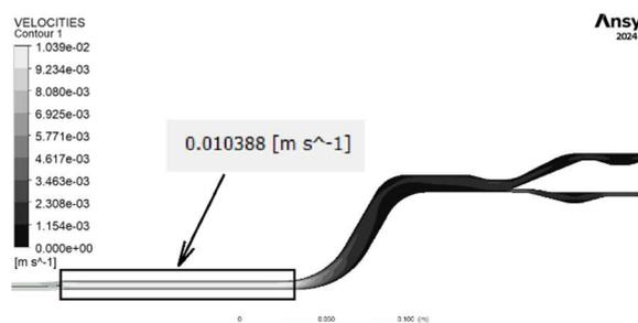
**Figure 6** - Distribution of PP melt flow velocity in the head (0 wt% MWCNTs)
