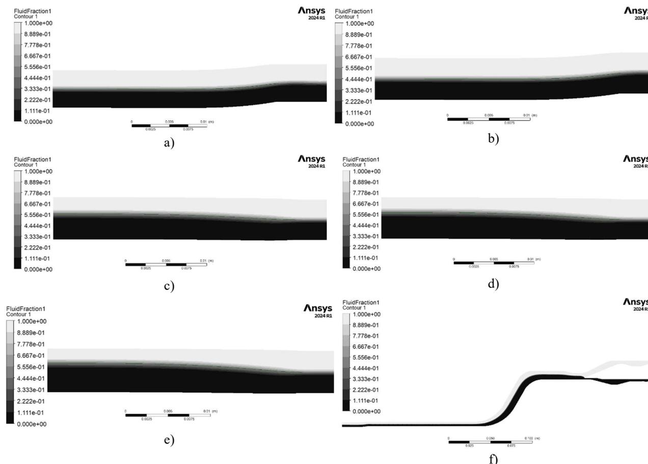
**Figure 11** - Thickness distribution of PVC (black) and PP/MWCNT (white) layers at different MWCNT concentrations: (a) 0%, (b) 1%, (c) 2%, (d) 4%, (e) 8% and (f) 0%
