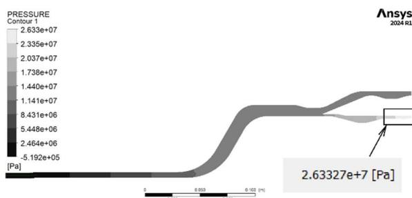
**Figure 5** - Pressure distribution in the extrusion head (0 wt% MWCNTs in PP)
