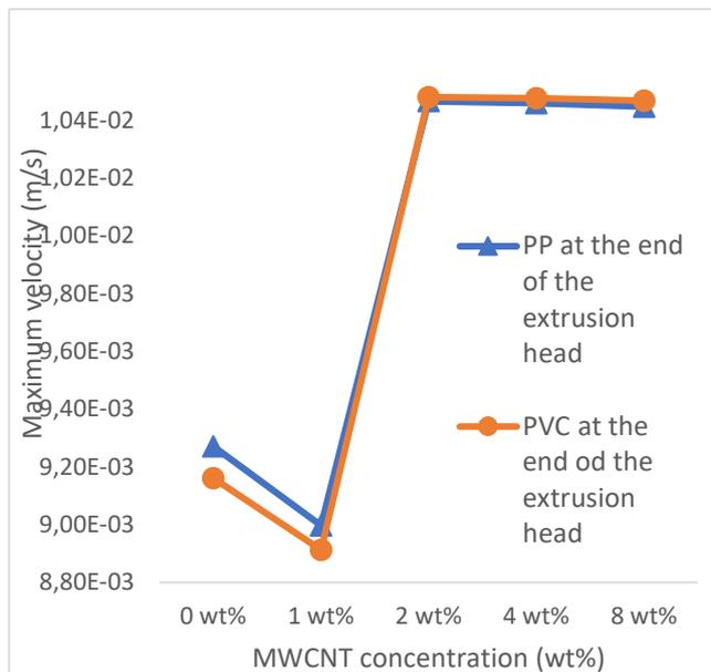
**Figure 9** - Dependence of maximum flow velocity of PP/MWCNT and PVC layers on MWCNT concentration at the end of the head
