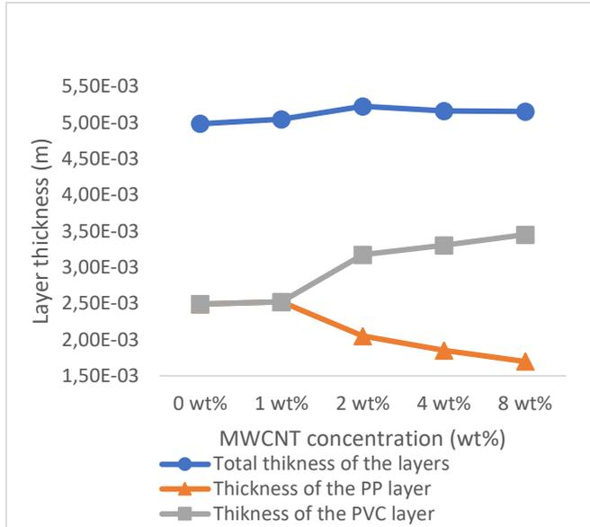
**Figure 7** - Dependence of extrudate layer thicknesses on MWCNT concentration
