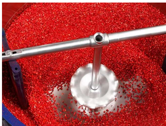
Fig. 4 – Photo of the multi-coater Petkus/Roeber rotating bowl [16]
